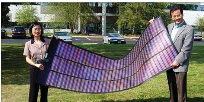
Dr. Deng and Xunlight co-founder Dr. Liwei Xu, showcase their flexible and lightweight photovoltaic panel.
